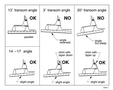
Figure 2-9: Transducer Angle Adjustment
